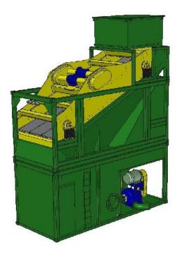
The SD2400DP Primary Shaker is a high capacity, steeply declined, single deck, linear motion shaker with up to 4 No. Metso MM200 centrifugal discharge pumps. The unit is used for the primary separation of gravels, coarse particles or clay balls. The SD2400DP consists of a shaker module mounted on top of a 20' container sized pump tank module plus up to two free-standing discharge pumps.
