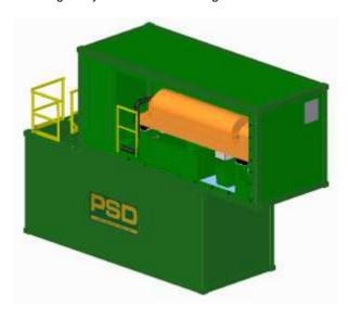
The S3-01-H consists of two modules, each 6058x2438x2591mm high being the size of a standard 20 foot, type 1CC freight container, complete with ISO corner castings. In operation the centrifuge module mounts on top of the power-house module, so that the complete machine requires a working footprint of 7.9m x 2.5m and stands 5.2m high. The centrifuge is fed by a variable speed pump system. The rate of fluid feed to the centrifuge is controlled by altering the speed of the feed pump.
